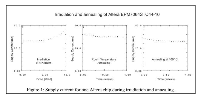
Exactly the same pattern of supply current was seen for all 16 Altera chips. For the Exar chips the supply currents were constant throughout all phases of the test. In ATLAS the dose rate is very low and the annealing process occurs continuously. Thus no increase in supply current is anticipated. Annealing is recommended as part of the test procedure in MIL-STD-883E, Method 1019.5 to account for low dose rate effects.
