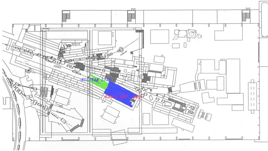
Figure 2.2: The lay out of the East Hall at KEK. The E391a experimental area is the shaded region in the center of the figure and the PI0 beam-test area is below and to the left on the diagram.
