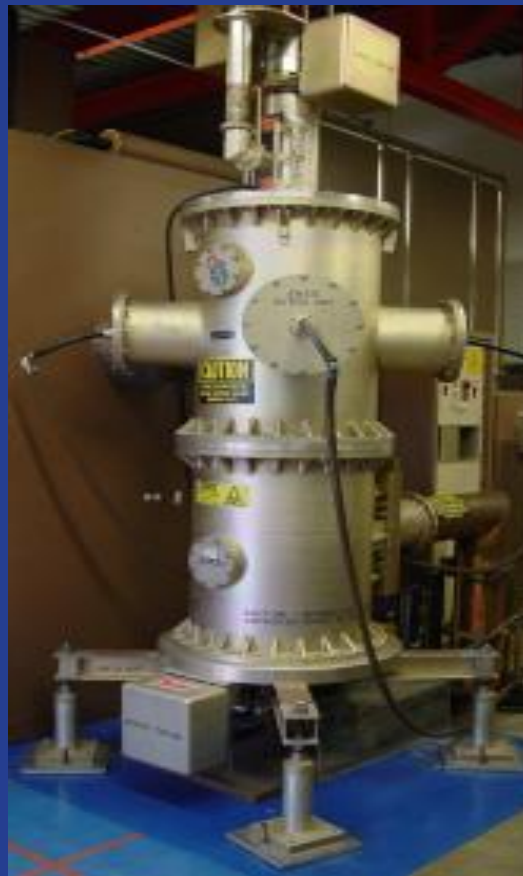
200 MHz Alvarez LE DTL Accelerating Cavity
