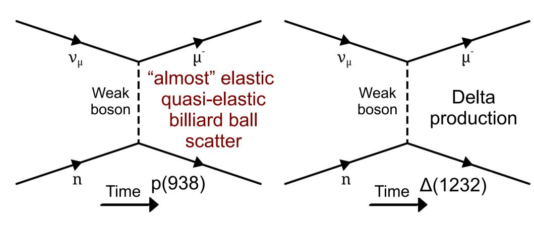
Today's results focus on the kinematics from the quasi-elastic to Delta resonance interactions. not the only topic, but very important for NOvA, T2K, DUNE. Will refer to W as the (invariant) mass of the outgoing hadron. QE has just a proton 0.938 GeV, Δ has 1.232 GeV
