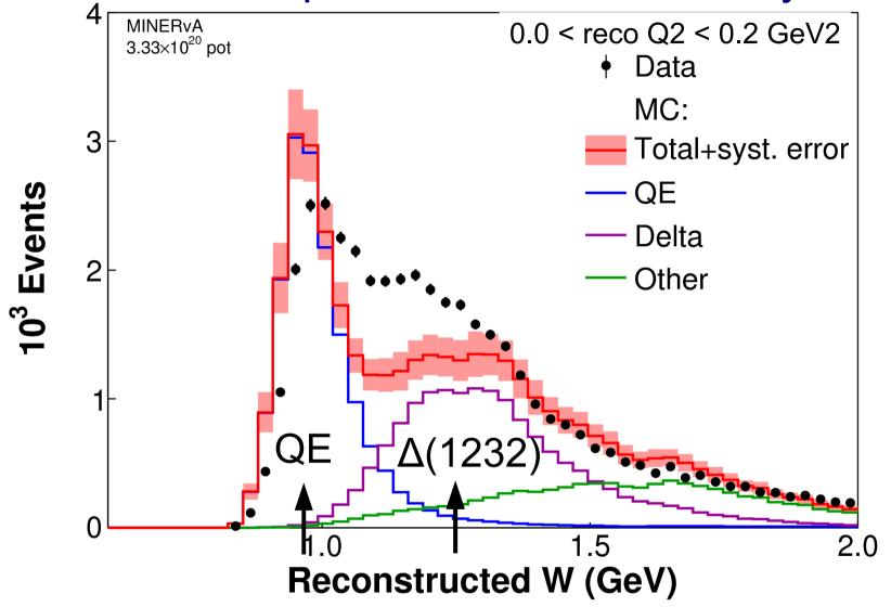
Fully simulated GENIE + MINERvA tuned pion (GENIE is the name of a neutrino interaction computer code) something is funny about the QE and the data might have a 2p2h process in the dip
