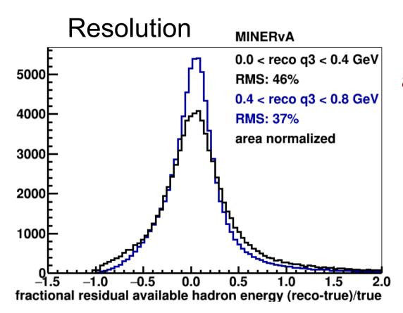
Use known resolution to "unfold" reconstructed data (similar image processing to unblur a photograph)
