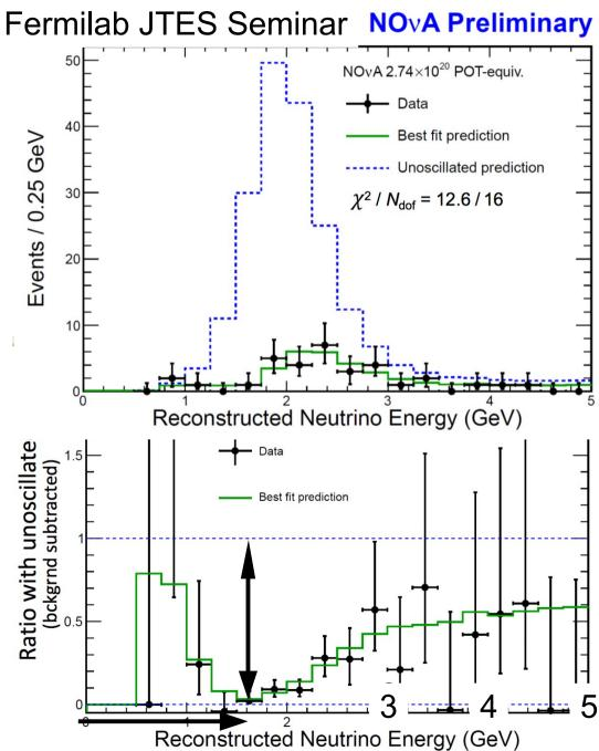
Extraction of oscillation parameters comes from comparing predicted energy spectrum with no oscillations to the measured ones, and fitting parameters.
