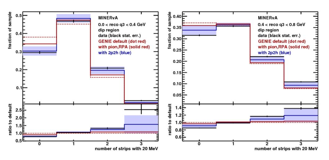
Easiest to focus on the ratio plot at the bottom, 2 and 3 protons. The 2p2h model is shifted much closer to the data. Without 2p2h, poor description of the data,  $\chi 2 = 15.1$  for 6 dof Data want more 2p2h, or use all the error band,  $\chi 2 = 7.5$
