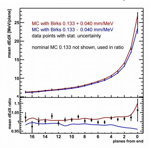
(above) dEdX trend compared to nominal 0.133 ± 0.040 mm/MeV (right) profiles for individual points actually used to do the fit shown at best fit 0.0905 ± 0.015
