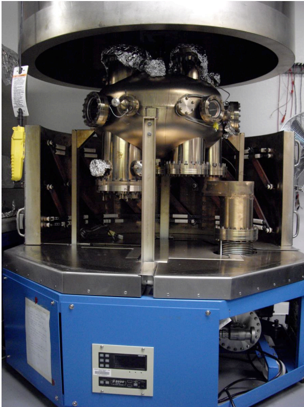
Fig. 7. Large ultrahigh vacuum process tank capable of accommodating 10" photocathodes at SSL.
