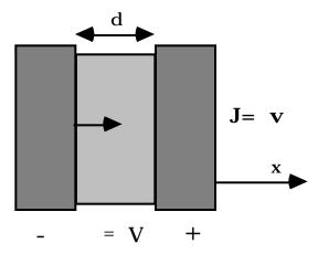
The arrow shows the direction of motion of the accelerated electrons. Assume the system can be treated as one-dimensional, that is the gap distance d is much smaller than the plate width. Assume that the flow is static, with no parameters changing in time. All of the electrons will have the same velocity v (in the x-direction) at given point in x.
