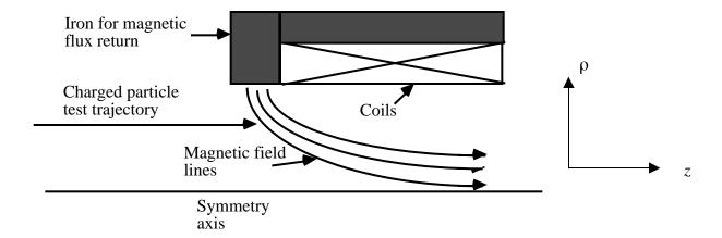
**Exercise 2.** In order to help you derive Busch's theorem, we refer to the figure above. The radial fringe field crossed with the longitudinal particle motion gives rise to an angular kick. This field can be approximated through use of Ampere's law
