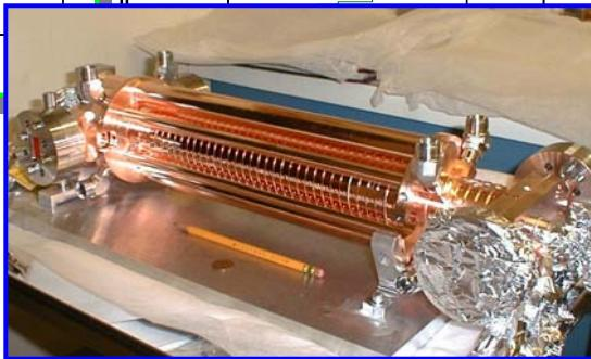
0.6-m section, 22 MV available at SLAC (200- $\mu\text{m}$  alignment)
