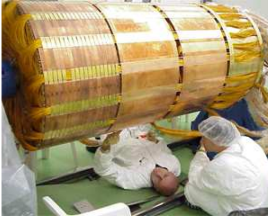
Figure 5.23: Assembly of FCal modules: from left to right, the three modules plus the copper alloy plug can be seen on the support mandrel with most of the cabling in place.
