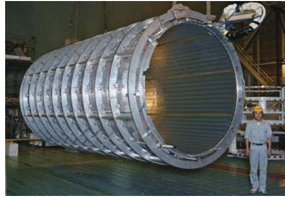
Figure 2.2: Bare central solenoid in the factory after completion of the coil winding.
