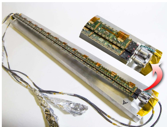
Figure 4.5: Close up of a bi-stave loaded with modules. The insert shows the U-link cooling connection between staves.
