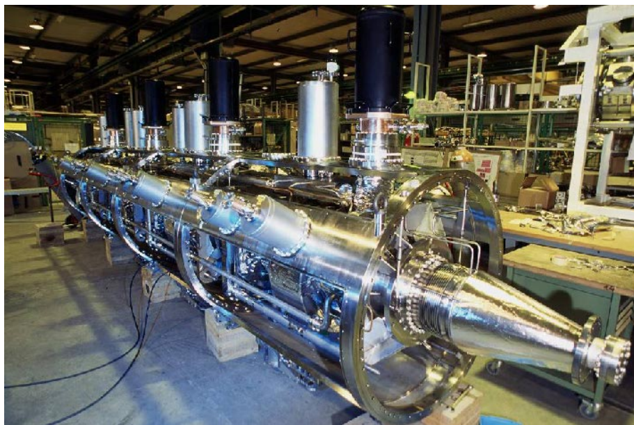
Figure 4.2: Four-cavity module during assembly.
