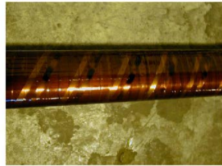
Figure 5.6: Wrapping of the stainless steel strips as bakeout heaters and a close up view of a finished chamber before the addition of the aluminised layer.
