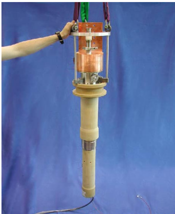
Figure 6.5: 13 kA CERN prototype HTS current lead.
